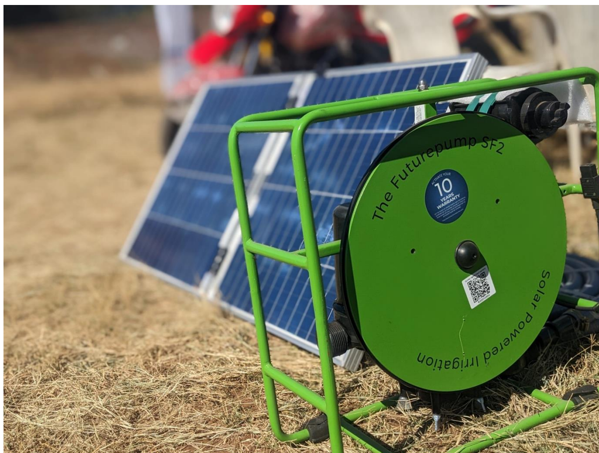
Figure 3.90: Solar Irrigation pump
